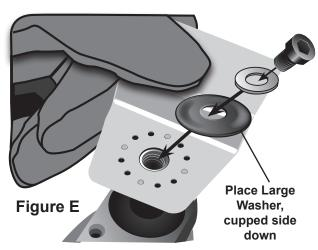
3. Slide the Small Washer (2), then the Large Washer (3) onto the the Cap Screw (1). Make sure the cupped side of the Large Washer is toward the tool. While holding the attachment over the pins on the tool, thread the Cap Screw in place. (See Figure E.)
